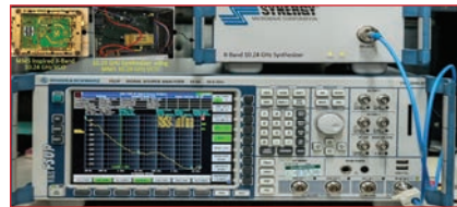
▲ Fig. 2 Phase noise measurement setup for the 10.24 GHz synthesizer using MMS inspired oscillator.
